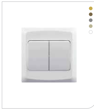
C304W 10Amp 2 gang 2 way switch (wide dolly) 86.5 x 86.5mm
