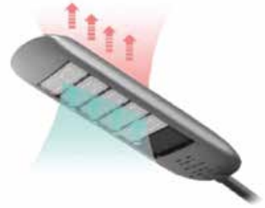
Schematic diagram of heat dissipation of honeycomb effect
